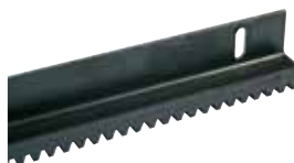
ACS9040 Module 4 RACK in iron (sect. 22 x 22 mm) with right-angle member (up to 2200 kg) recommended for K500 FAST in 2 m bars per m
