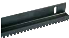
ACS9050 Module 4 RACK in iron (sect. 22 x 22 mm) with CATAPHORESIS treatment, right-angle (up to 2200 kg) recommended for K500 FAST - in 2 m bars per m
